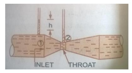
As pipe is horizontal,  $z_1 = z_2$  and  $\frac{P_1 - P_2}{\rho g} = h$ , where h is the manometric head which is equals to difference of pressure heads between two sections.
