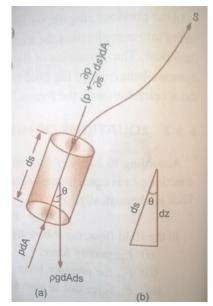
The resultant force on the fluid element in the direction *S* must be equal to the product of mass of fluid element and acceleration in the direction *S*.
